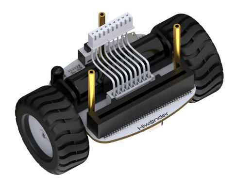
Step 5: Insert the flat cable into the upper plate.
