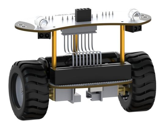
Step 6: Fix the upper and bottom plates together with another three screws.
